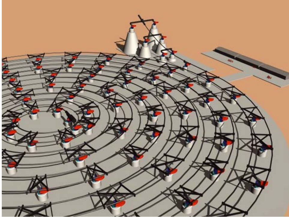
FIGURE 8. Illustration of a Spiral Slingatron in which a 1 ton Projectile is accelerated around a 12-turn Spiral of Outer Radius 160 meters to a Speed of 9 km/sec.
